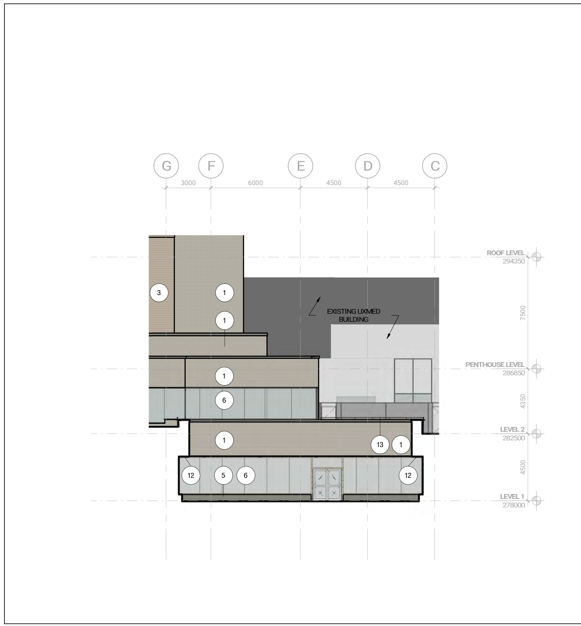
COURTYARD ELEVATION LOOKING EAST ref. 1 / A672 1:150 A301.5
